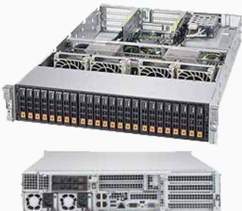
Figure 12: Supermicro's 2028U-TN24R4T+ with 24 x NVMe bays in a 2U chassis
