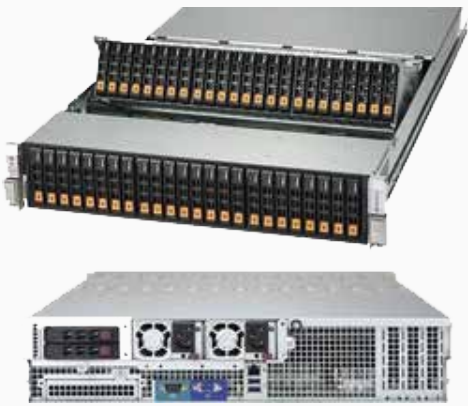
Figure 13: Supermicro's 2028R-NR48N with 48 x NVMe bays in a 2U chassis.
