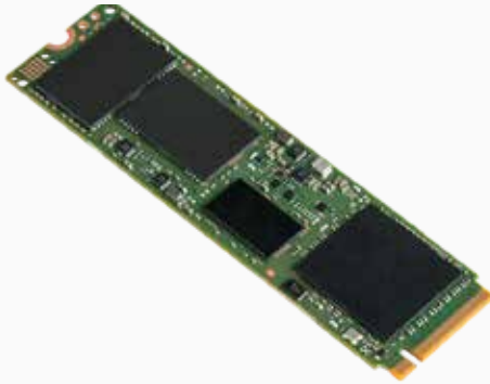
Figure 6: Intel P3100 M.2 NVMe device
