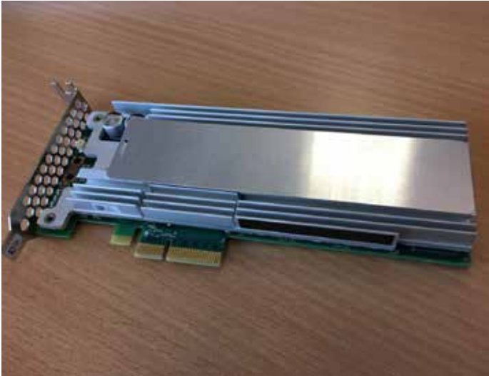
Figure 1: Intel P3700 PCI-Express x4 NVMe device
