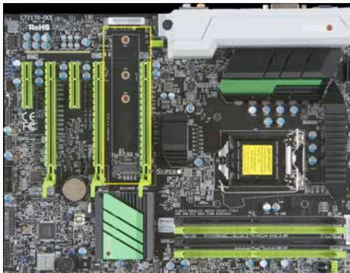
Figure 7: Supermicro C7Z170-OCE motherboard supporting M.2
