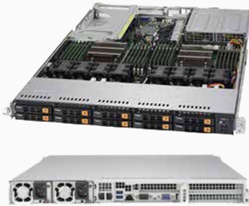
Figure 11: Supermicro's 1028U-TN10RT+ with 10 x NVMe bays in a 1U chassis
