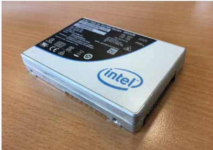
Figure 2: Intel D3700 U.2 Form Factor NVMe device
