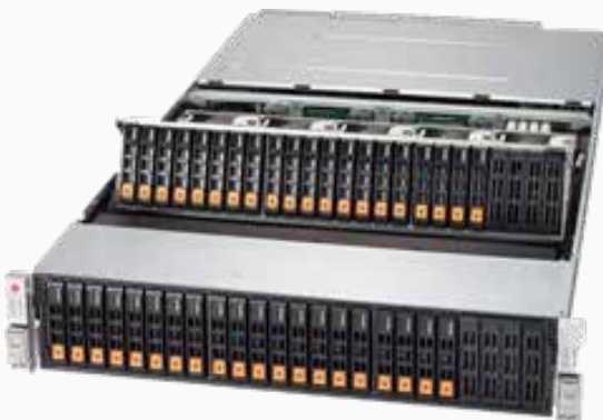
Figure 14: Supermicro's SSG-2028R-DN2R40L with 40 x NVMe and dual x86 systems in a 2U
