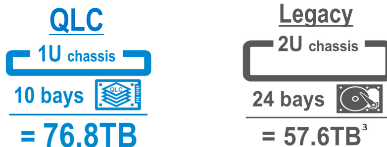
Figure 1: Maximum raw capacity (1U chassis with QLC, 2U chassis with legacy HDDs)
