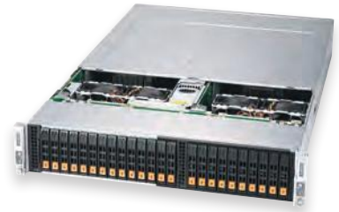
Dual DP Nodes, 24 Hybrid NVMe/SAS3 Drive Bays
