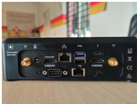
Rear (left to right): Wi-Fi antenna port, Power, Protected UHD HDMI, VGA, 2x RJ-45, USB 3.1 Type-A, USB 2.0 Type-A, Thunderbolt 3, HDMI, Wi-Fi antenna port.
