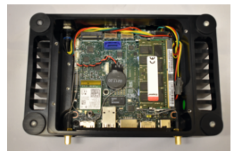
The Intel Wireless AC 9260 Wi-Fi card can be easily replaced.
