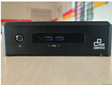
Front (left to right): Power, 2x USB 3.1 Type-A.
