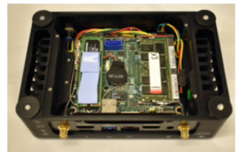
Full-length M.2 2280 SSDs can be installed.
